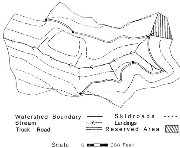
Figure 1.-An example of a forest road system meeting West Virginia Best Management Practice standards. It was used to remove approximately 1/2 million board feet of timber from a 96-acre Appalachian watershed.
