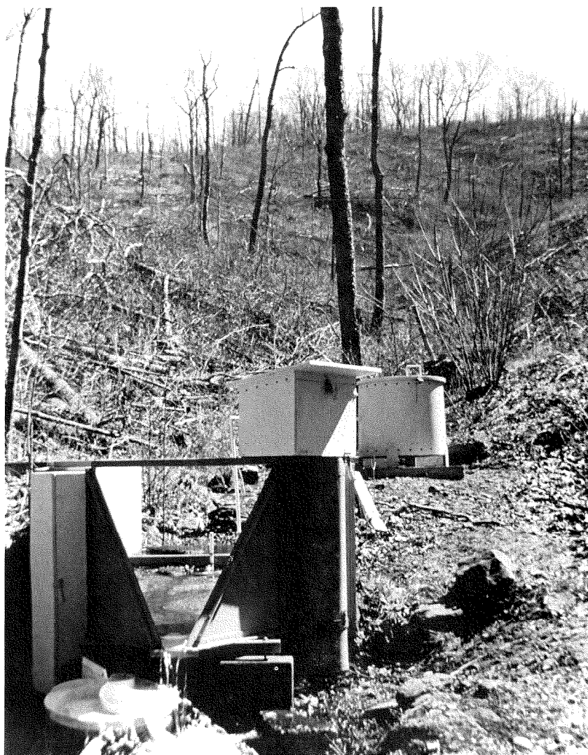
Figure 1 -Streamflow increases after clearcutting as shown by this gauging station in a Clearcut watershed.
